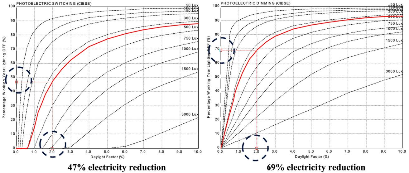
Fig. 11. Virtual sensor system for electric lighting: on-off mode (left), dimming switch mode (right) for East orientation, 30% WWR per office.
