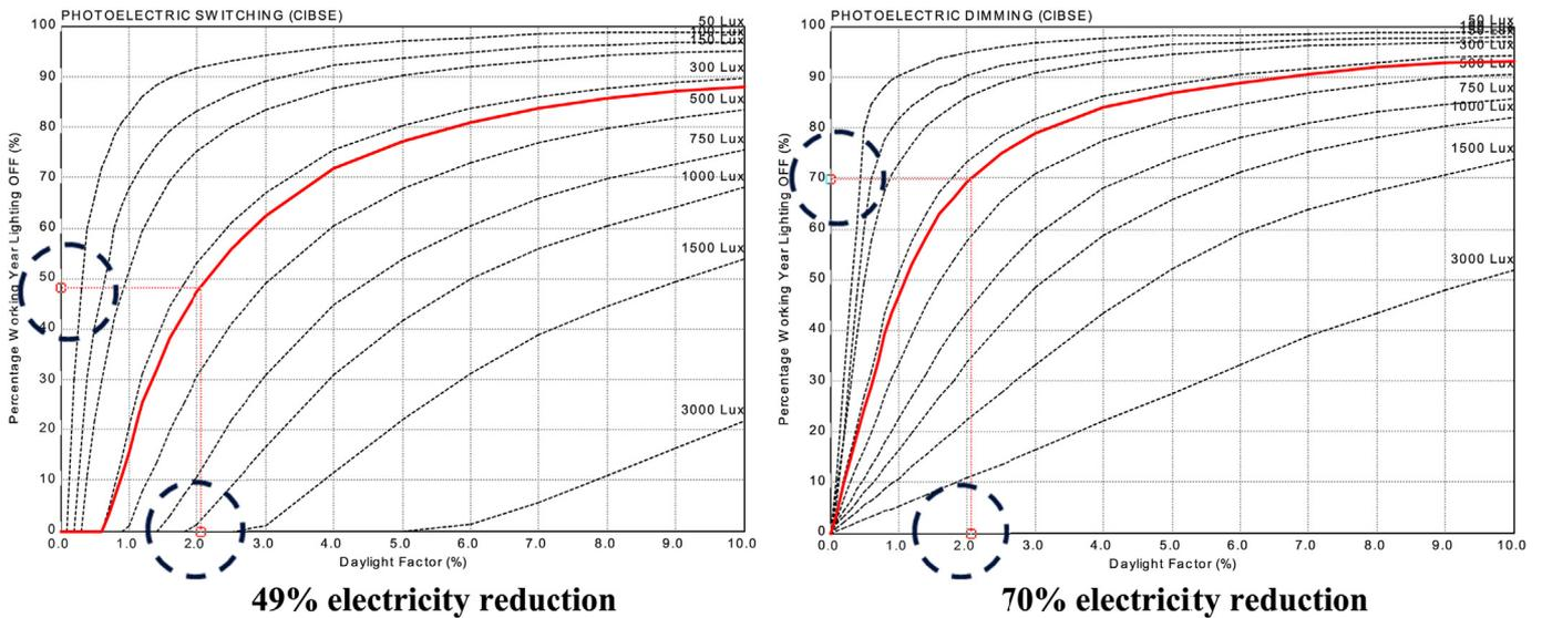
Fig. 12. Virtual sensor system for electric lighting: on-off mode (left), dimming switch mode (right) for South orientation, 25% WWR per office.
